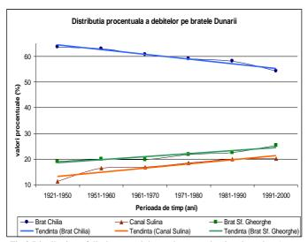
Fig.2 Distribution of discharge and the tendency on the river branches (processing after Bondar, 2004; Gâștescu, Driga, 2008)
